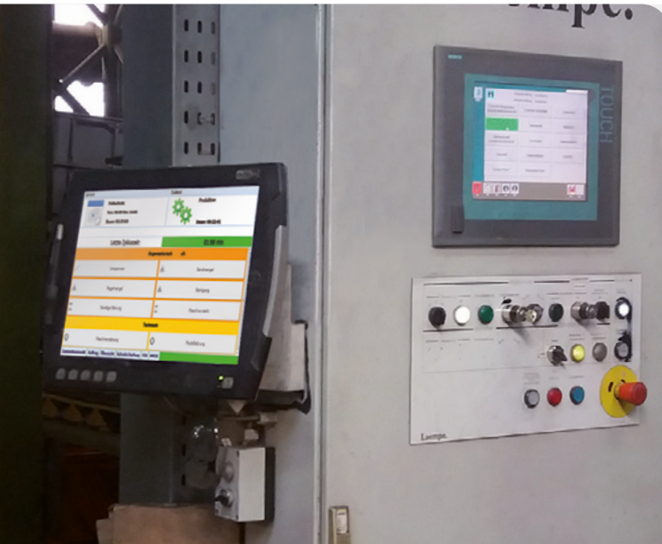
Reasons for downtimes can be selected directly at the core shooting system by touch.
